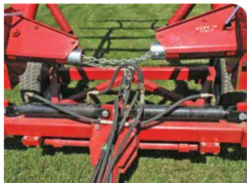
Hydraulic cylinders and hoses supplied.
