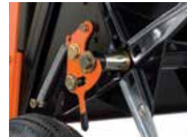
SmartLINK™ system patented locking device enables attachments to lock in and unlock in seconds.
