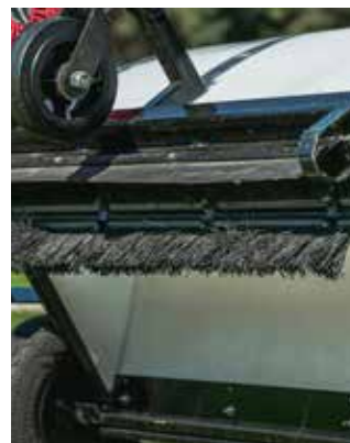
Long-life nylon brushes to withstand continuous use.
